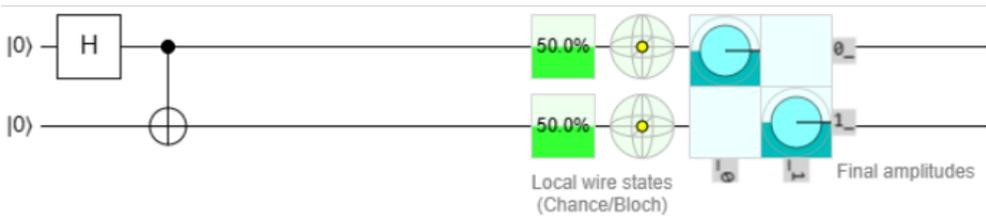
**Figure 3.** An example of a circuit for obtaining an entangled state. The initial state of the system is  $|00\rangle$ . After applying the Hadamard  $H$  gate, we will get the state  $\frac{1}{\sqrt{2}}(|00\rangle + |01\rangle)$ . Then, when the CNOT gateway is applied, the state changes to  $\frac{1}{\sqrt{2}}(|00\rangle + |11\rangle)$  which is an entangled state (it cannot be represented as the product of two states). Source <https://algassert.com/quirk>.
