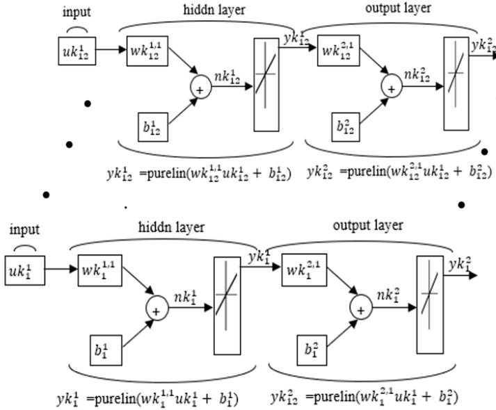
**Figure 5.** The idea of the architecture of neural networks. Source: own elaboration based on [1].
