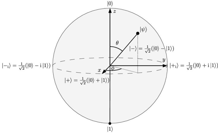
**Figure 1.** Bloch Sphere, z-axis represents the base quantum state of  $|0\rangle$  and  $|1\rangle$ , x - axis represents Hadamard state, y-axis represents the base of complex component. Source [6].
