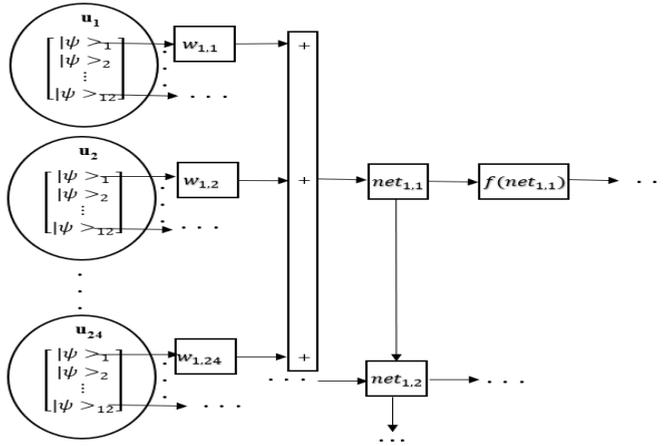
**Figure 4.** Example of processing mixed quantum states for the hidden layer for the first qubit for the first neuron. Symbols:  $f(\text{net}_{1,1})$  - activation function,  $\text{net}_{1,1}$  - the value of the weighted sum of the input signals of the first quantum state,  $w_{1,n}$  - weight density matrix,  $|\psi\rangle_n$  -  $n$ -th quantum mixed state. Source: Own elaboration.
