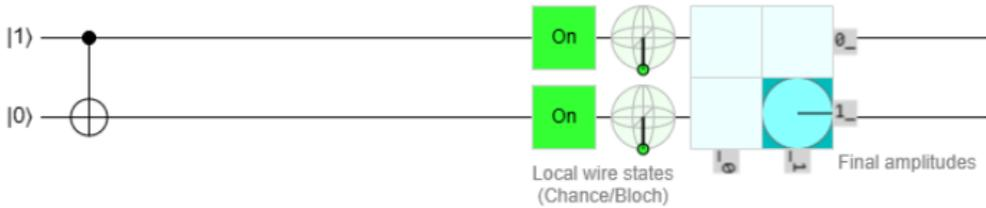
**Figure 2.** Example of how a CNOT gateway works on a two-qubit state  $|10\rangle$  (left side) transform on  $|11\rangle$  state (right down corner). Source: own elaboration on the site <https://algassert.com/quirk>.
